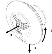
To refit the cover, reverse the above procedure. If when refitting the front cover the iris stays open, remove the cover and don't attempt to refit it for approx. two minutes (allowing the actuator to retract back in the closed position). Then try again.
